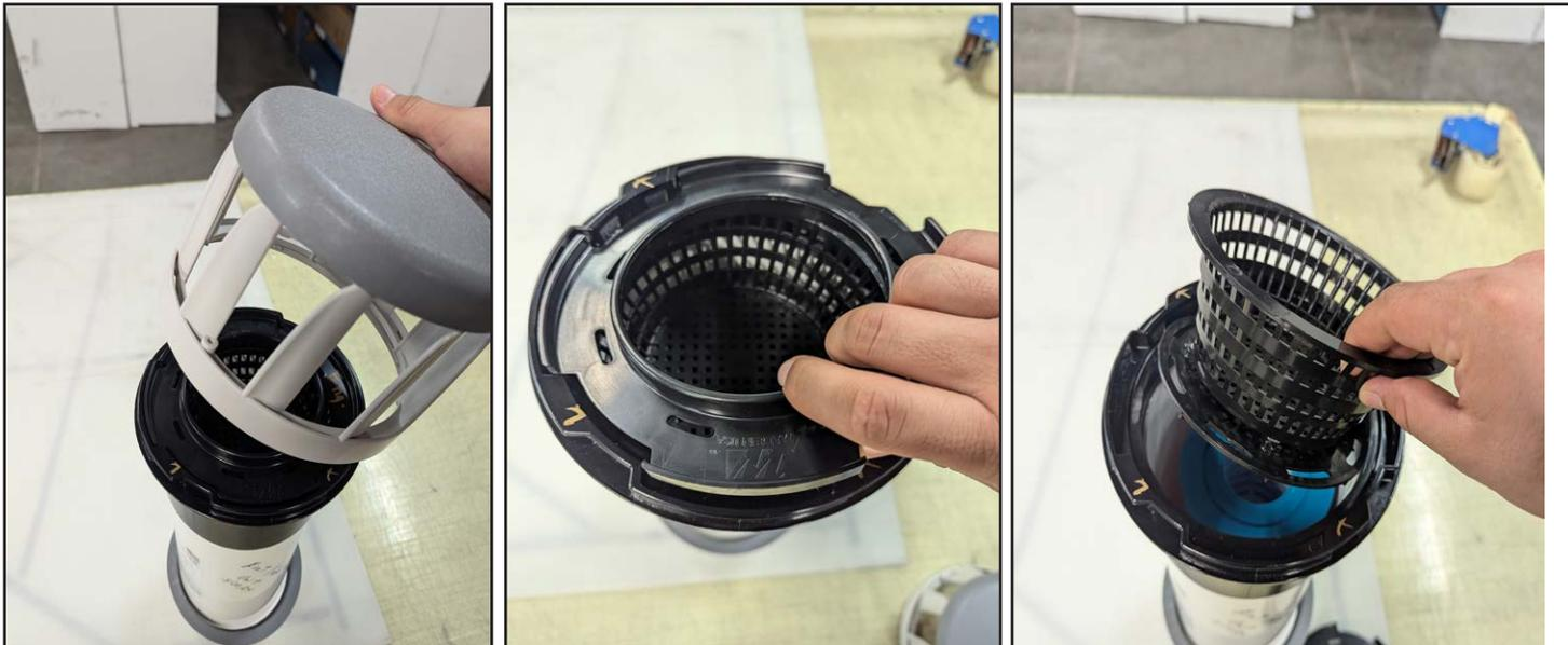
Note: Always fill the spa through the filter canister. This will help prevent air pockets from forming inside of the plumbing. Air pockets will prevent the primary pump from operating properly.
