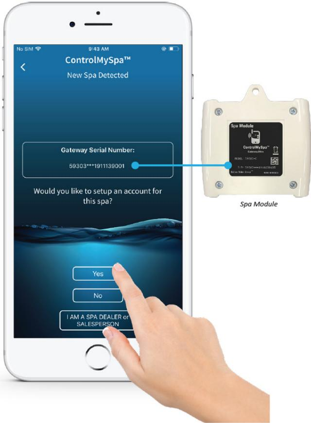
5- The App will begin scanning for the spas wifi module. within a few seconds the module serial number should appear.
