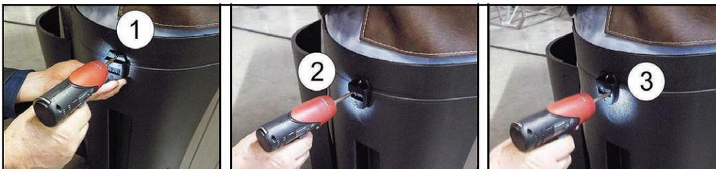
**Step 4** Use a screwdriver to finish screwing in the three screws, repeat this process for the remaining 3 corners.
