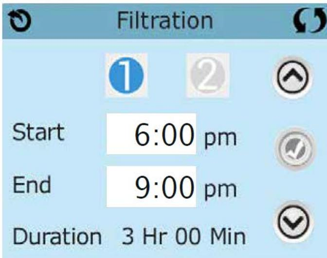
Viewing Filter 1 while Filter 2 is OFF:
